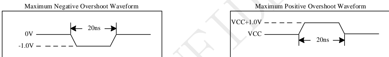
Figure 5-2 Input Test Waveforms and Measurement Level
